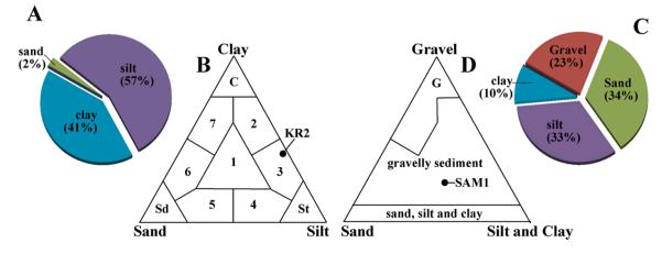
**Fig. 5.** Grain size analysis on raw materials and the Shepard (1954) classification ternary diagrams for samples KR2 (A-B) and SAM1 (C-D). In ternary B: C = clay; St = silt; Sd = sand; 1) sand, silt and clay; 2) silty clay; 3) clayey silt; 4) sandy silt; 5) silty sand; 6) clayey sand; 7) sandy clay. In ternary D: G = gravel.
