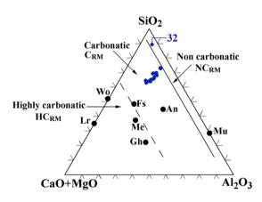
Fig. 6. Ternary diagram illustrating the distinction between non-carbonatic, carbonatic and highly carbonatic ceramic bodies.
